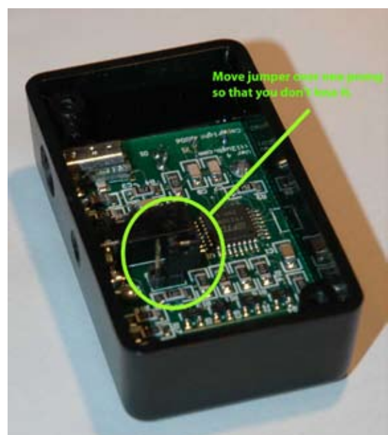
Open jumper, separate transmit and receive lines. Use for FT-857, 897, etc
