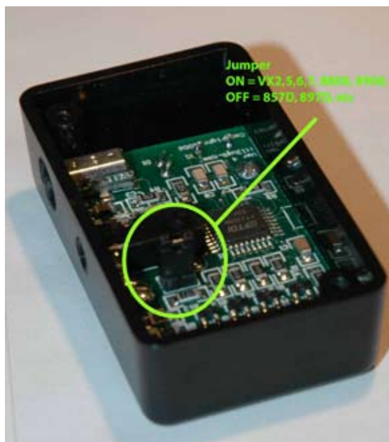
Stock Configuration, combined transmit and receive lines. Use for VX-2R, 5R, 6R, 7R and FT-8700, 8800, 8900, etc.
